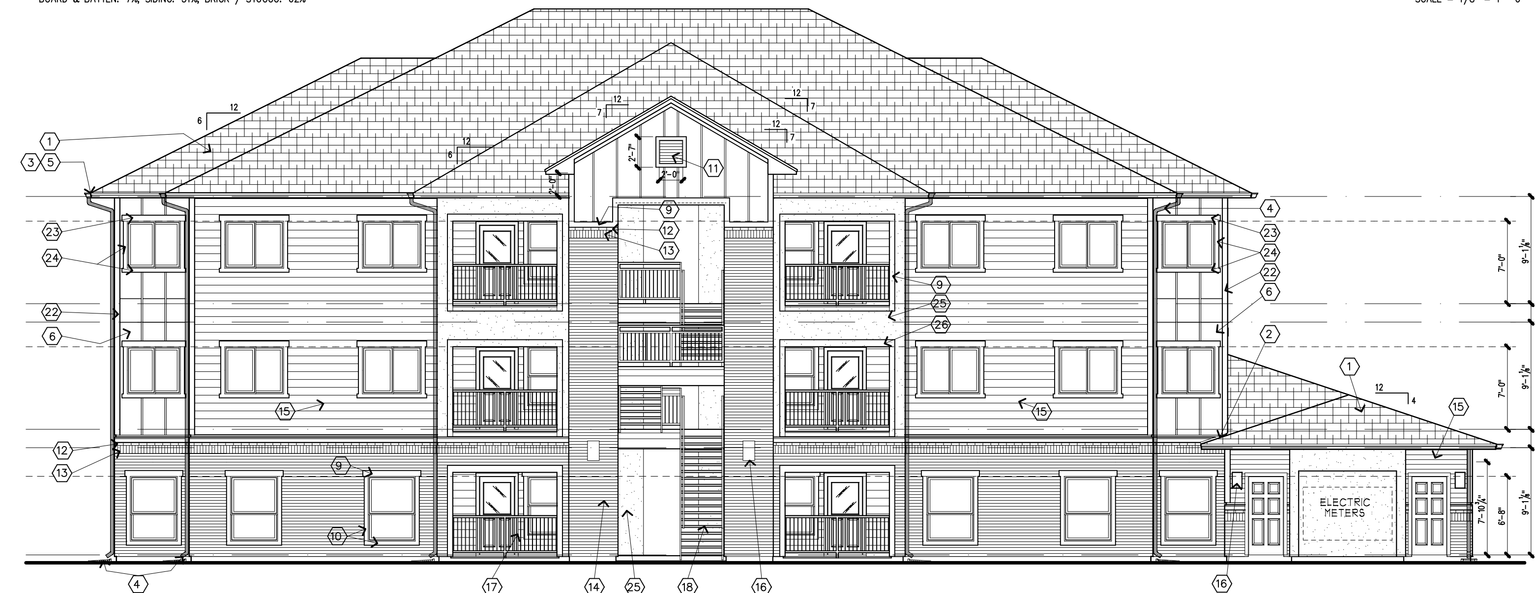
BUILDING TYPE IV - WEST ELEVATION
