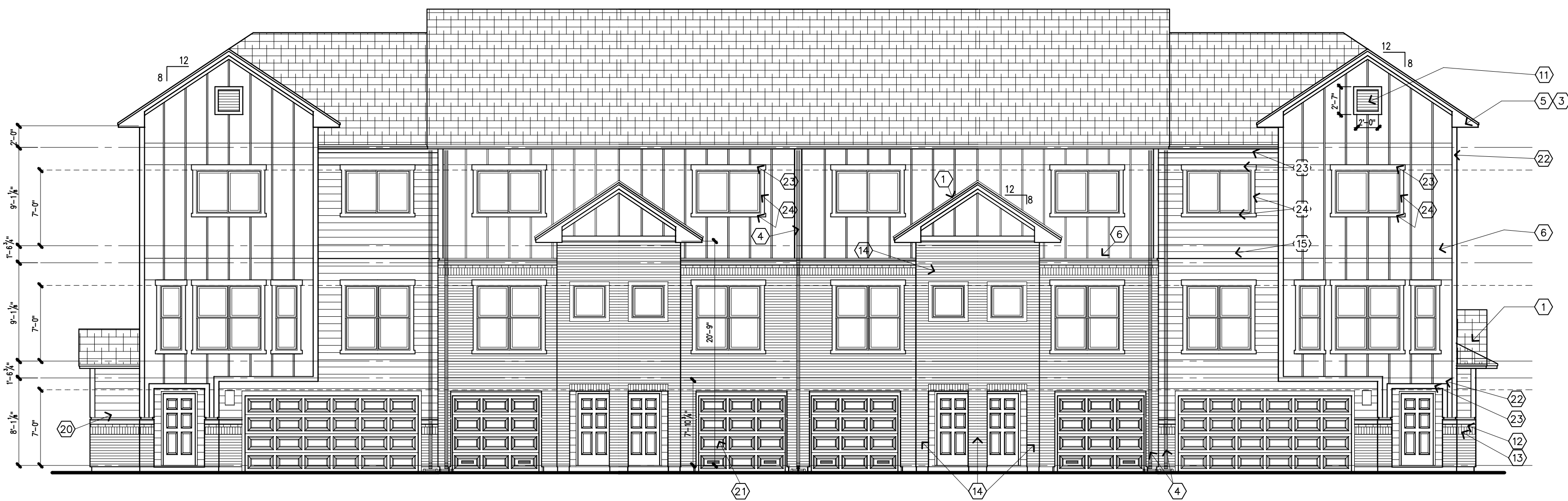
BUILDING TYPE T1 WEST ELEVATION
