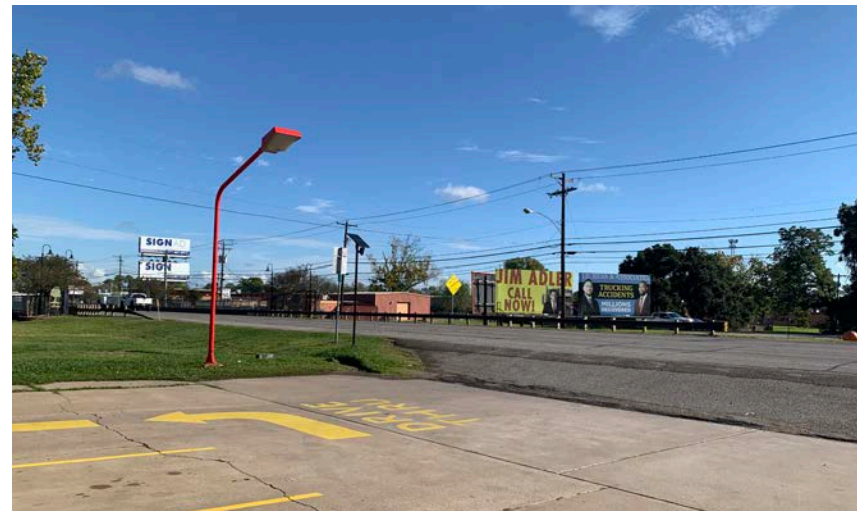
Photo taken north of N. Gordon Street. No sidewalks on either side of the bridge crossing. The slope from the right of way connecting to neighboring properties is too steep both for vehicular and pedestrian/cyclist usage.
