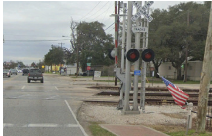
➡ This photo shows the sidewalk abruptly stops leading up to the crossing, and uneven shoulder width at the crossing.
